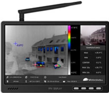
Workswell WIRIS can be fully controlled using a traditional RC controller from which all functions of the system are accessible. In addition to all functions, the monitor displays images from the thermal camera as well as the colour camera.
