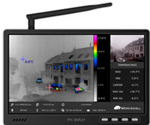
*Workswell WIRIS can be fully controlled by a traditional RC controller from which all system functions can be accessed. In addition to all functions, the monitor displays images from the thermal camera as well as colour camera. Information is available about the measured temperature (min/max and central spot) during the flight.*
